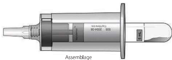
Figure 5.5 Loading of the vacutainer bottle into the tube holder.
